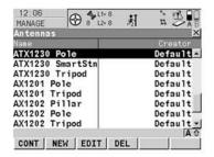
In the Name type in your description. In this instance we have used Bathymetric. Do not change other settings. In the IGS Screen change. IGS Name. Serial Number. Set Up Number. This gives your set up a unique IGS. Command: Store. Antenna is now set up: Note Antenna height must be set later!
