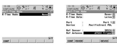
Set your required radio channel. This can be changed later if the channel is unavailable or corrupt Command: Cont. Set the Antenna that you have already set up by toggling the arrows. Ensure that the Default HT & Moving Ht are set to the dimension from the base of the transducer to the bottom of the antenna. Command: Cont.
