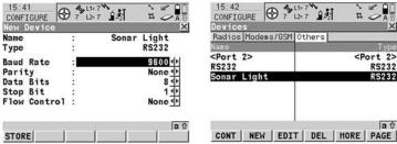
Type in your Name. We have used Sonar Light. Set the Rates as above. See Sonar light manual page 14. Command: Store. The GPS will now receive Data from the Sonar light. Command: Continue.
