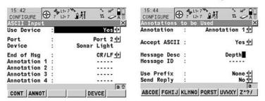
You must now set the end of message and Annotation 1. Command: Annot. Type in your Message description. We use Depth. Ensure the Accept ASCII is set to Yes. User Prefix is set to None. Send Reply is set to No. Command: enter.
