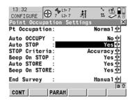
Create a new Template. Command: New. Create a new ID with sufficient logging point's we have set ours to a million as you may be collecting a lot of data. Increment by Numeric only. Command: Cont
