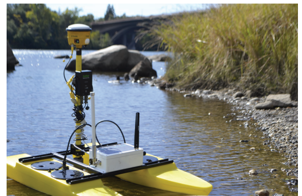
Unit can be integrated into remote / autonomous survey vessels
