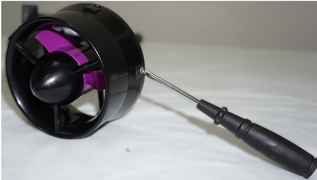
Figure 78: Thruster Housing Removal
