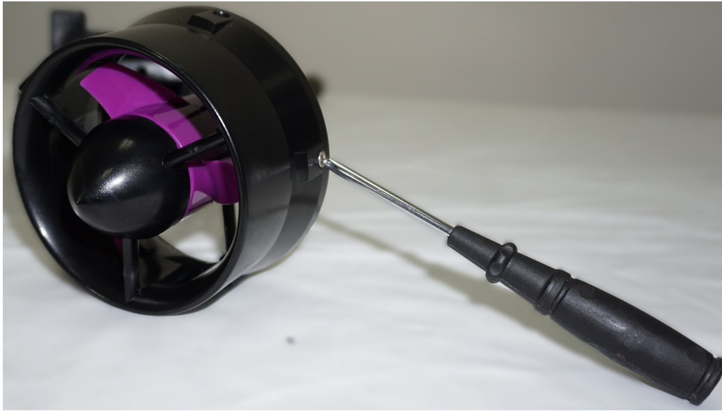
Figure 84: Thruster Housing Removal
