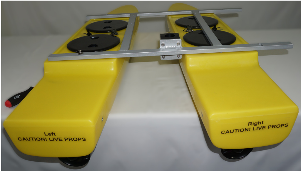
Figure 9: Pontoons Not Spaced Correctly
